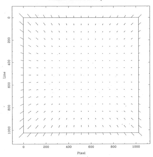
Figure 3. NAC distortion model. The corrections are sampled every 64 pixels and scaled up by a factor of 100.
