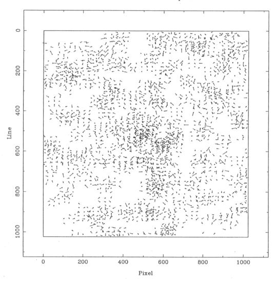
Figure 2. WAC postfit residuals. These are scaled up by a factor of 100 and plotted at the location of the image.
