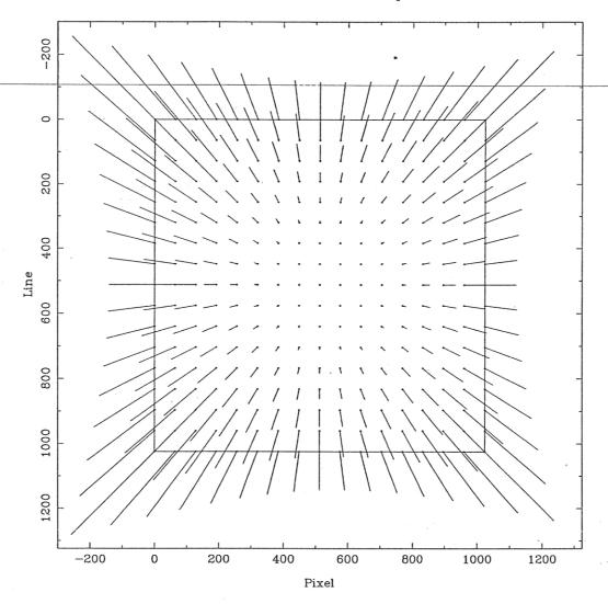
Figure 4. WAC distortion model. The corrections are sampled every 64 pixels and scaled up by a factor of 100. Note that the corrections in the corners are almost 3 pixels in each coordinate, and there is therefore more margin around the field of view in this figure.
